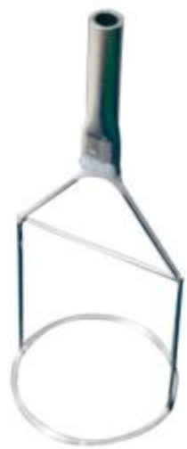
Platinum wire radius: 0.30mm Platinum ring radius: 9.85mm
